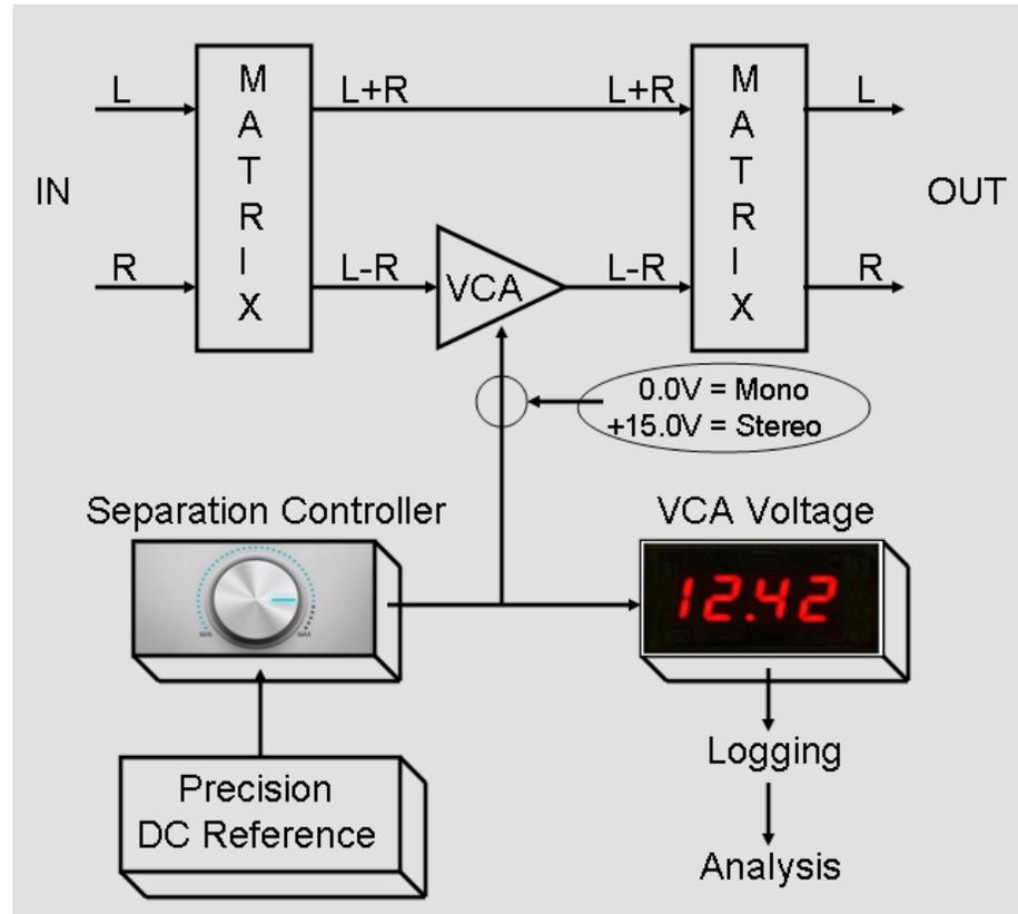
Fig 1 Stereo Separation Test Fixture
