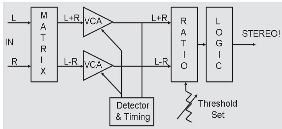
Fig 4 Autoranging Stereo Detector
